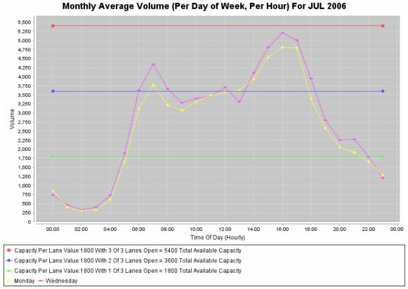
FIGURE 5 Capacity Volume Threshold Graph.
